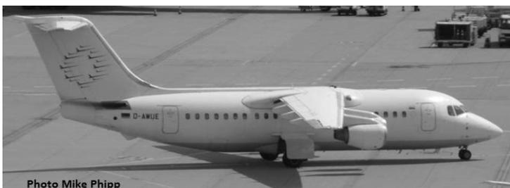
The wing was very 'clean' with the engines on pylons enabling large and long flaps without the need for leading edge slats with the benefit of minimal pitch change avoiding the complication of a moving tailplane. The addition of tail-mounted speed brakes further aided short field performance.
